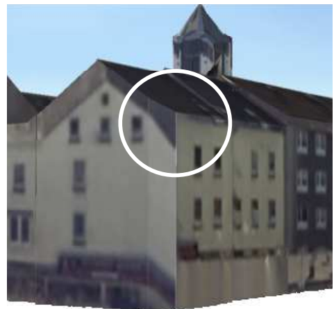
Figure 23: Shift of texture (left facades do not reach to the roof, right facades do match) indicate model’s precision.
