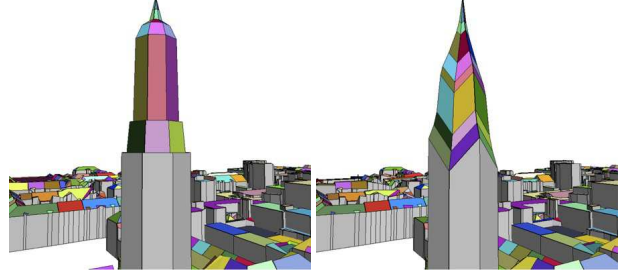
Figure 16: If one chooses \mu as a bound for height changes and does not consider rounding errors of x - and y -coordinates, then linear optimization changes the shape of the tower (from left to right) [1].
