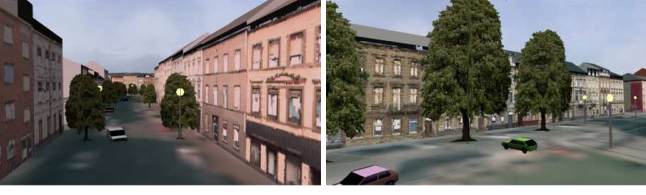
Figure 17: Texturing of facades requires higher precision of z -coordinates. Black areas between textures and roofs indicate that walls are too high whereas slopes of roof facets are too small [1].
