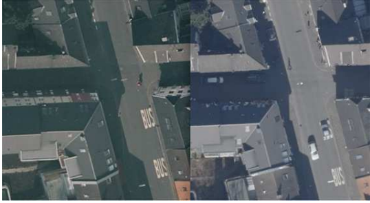
Figure 1: Orthophoto (left) vs. true orthophoto (right) [1]
