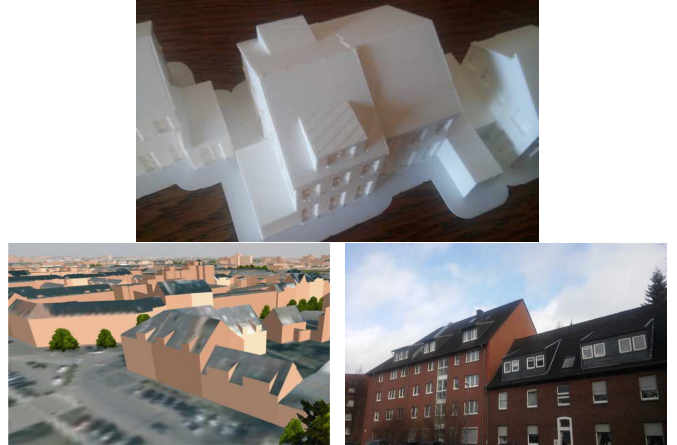
Figure 11: Top to bottom: 3D print of a building with rectangular dormers, a model with corrected rectangular dormers and the original buildings
